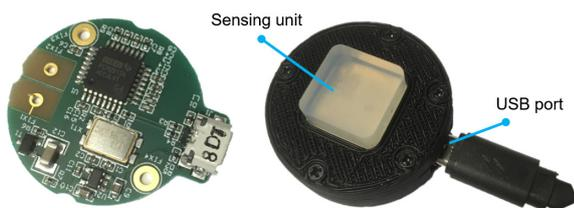
Figure 1: Electronic circuit board (left) of the system and assembled MICC device (right) with a USB cable connected.
