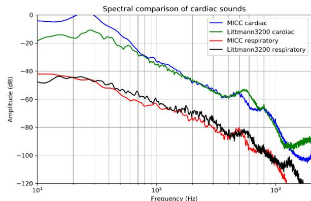
Figure 2: Spectral comparison of cardiac and respiratory sounds acquired by our device (MICC) and Littmann® 3200 stethoscope (amplitude of respiratory signals is decreased for visualization purposes).
