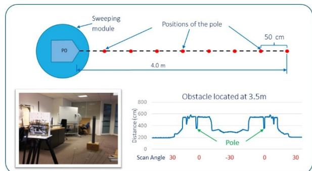
Figure 4: Test setup and results.
