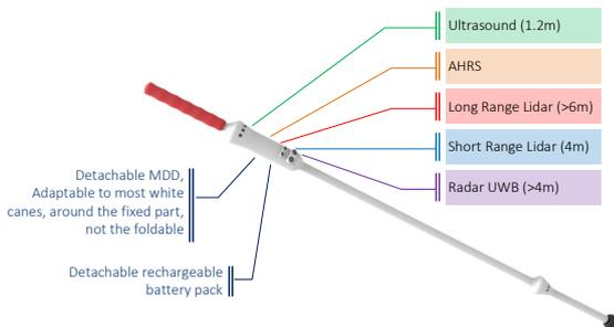
Figure 2: Projection of the final prototype to be implemented.
