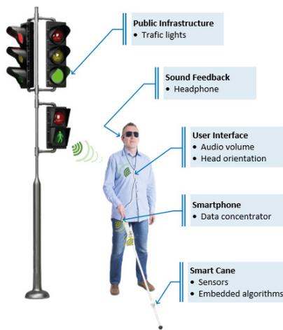
Figure 1: Full navigation system for the VIB.
