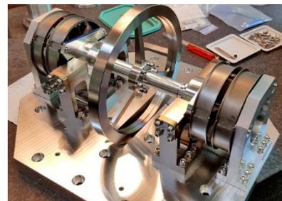
Figure 5: Vibration test bench with LAFP pivots assembled.
