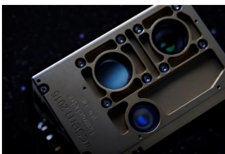
Figure 1: CSEM's VBN sensor. (top right) color camera optics. (bottom center) laser illumination head and above LiDAR receiver optics.
