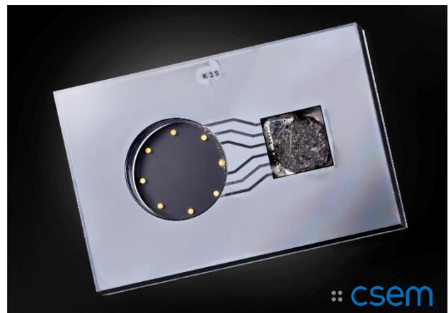
Figure 2: MEMS atomic vapor cell fabrication at the wafer level in CSEM's clean room facilities.
