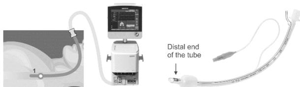
Figure 1: A printed pressure sensor for ventilation monitoring close to the lung at position 1 behind the balloon of the intubation tube.
