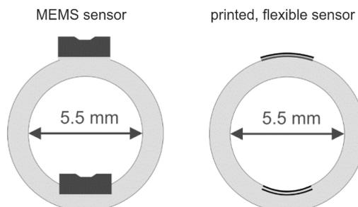
Figure 3: Cross section of a tube. Integration advantage of a thin, flexible sensor printed on polymer film.
