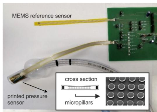
Figure 2: The prototype setup. A reference sensor and the printed sensor are mounted on an intubation tube and then put into a lung model to record different respiration cycles.
