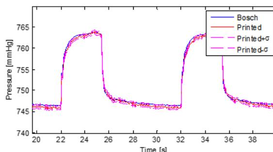
Figure 4: An example of the recorded respiration cycles. Here 1-sigma (deviation) of the pressure sensor is 0.42 mmHg. Recorded at UKBB.
