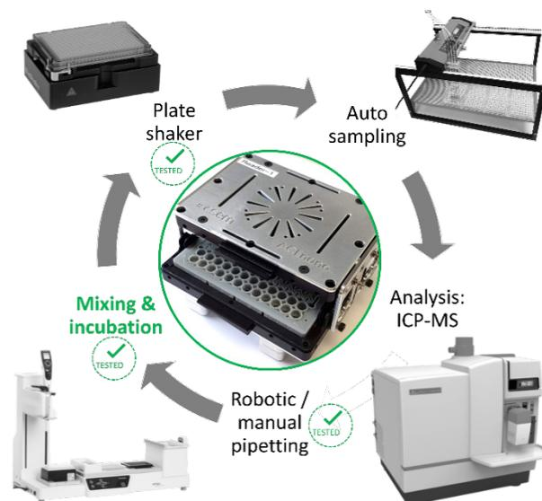
Figure 1: CSEM's automated sample preparation system (microfluidic chip inside the control unit) at the core of a new nanomaterial solubility assessment.
