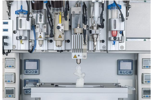
Figure 1: 3D discovery bioprinting platform from regenHU.
