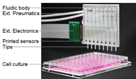
Figure 1: SenseCard on top a well plate containing a cell culture.
