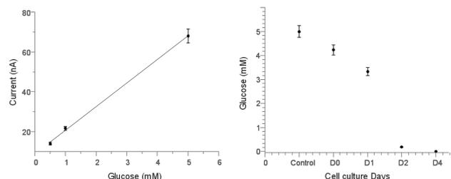
Figure 2: Electro-chemical sensor calibrated (left) and tested in cell culture over several days (right).
