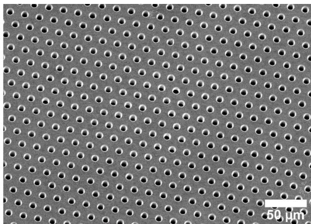
Figure 1: Metal membrane example (SEM micrograph).
