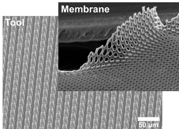
Figure 2: Example of a metal tool and the generated polymer membrane (SEM micrographs).
