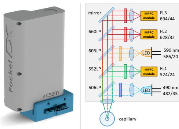
Figure 1: (left) Rendered view of the reader with microfluidic slide holder; (right) Optical sketch with spectral properties of filters and light sources.
