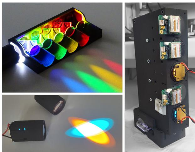
Figure 2: (top left) Optical setup with mounted spectral filters separating the light for the respective emission/detection channels; (bottom left) LED modules with cyan and orange light; (right) Reader equipped with light sources and detectors.
