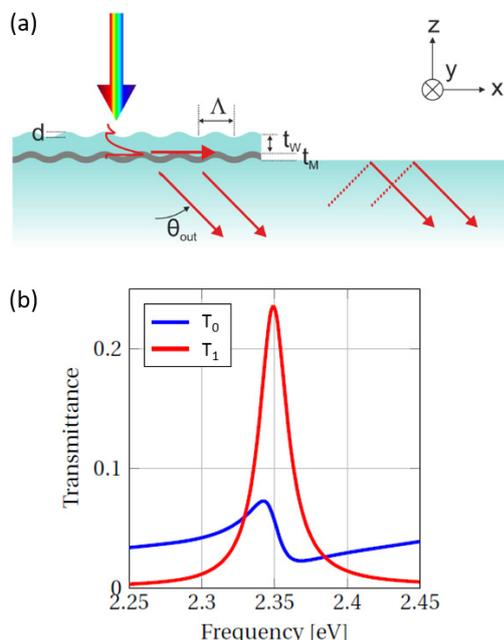
*Figure 1: (a) Wavelength selective coupling in a highly multimode light guide using a hybrid plasmonic-dielectric resonant waveguide grating. The incident light is coupled by grating diffraction into a hybrid surface plasmon-dielectric waveguide mode and released into the substrate. (b) The interference between the direct diffracted light and the light coupled into a waveguide mode yields a Fano interference in the zeroth and first order of diffraction.*
