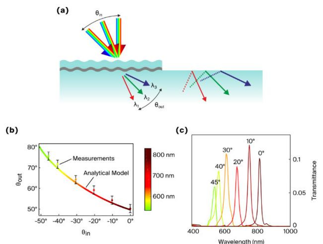
*Figure 2: (a) Diffracted angle and wavelength related to the diffraction peak as a function of dielectric waveguide thickness and the period. (b-c) Separation of incident white light with a large range of incidence angles into a set of quasi-monochromatic diffracted beams, comparison between measurements and analytical model.*
