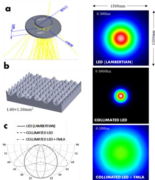
Figure 2: CSEM FMLA for uniform lighting. (left) FMLA 3D CAD model (top) and normalized (polar) luminous intensity distribution, LID (bottom; the Lambertian and the LID of the collimated incoming light are shown for comparison); (right) The corresponding Irradiance distributions over a 1'500x1'500 mm<sup>2</sup> planar detector located 1'000 mm away from the source; those produced by a Lambert and the collimated incoming beam are shown for comparison.
