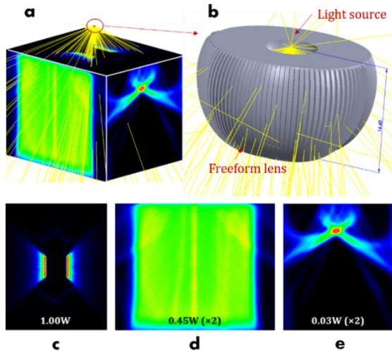
Figure 1: a) Uniform Irradiance distribution achieved using a freeform lens; b) designed at CSEM. The Irradiance distribution are presented and quantified in -c-, -d and -e.
