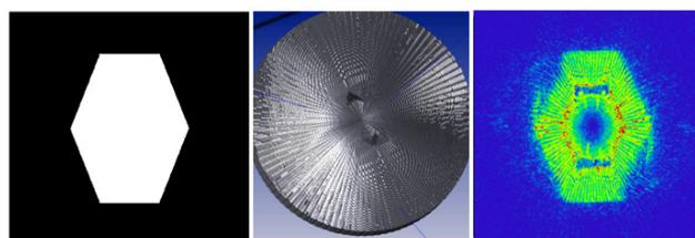
Figure 2: Left: Hexagonal target irradiance pattern. Middle: Designed freeform optical microstructures. Right: Irradiance pattern produced by the designed solution as predicted using raytracing software ZEMAX.
