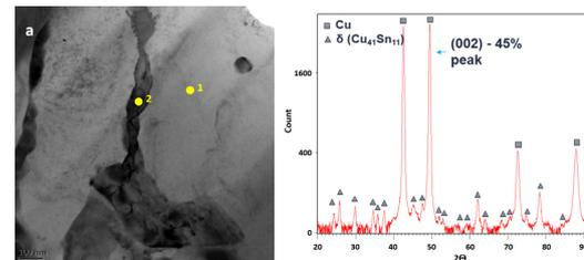
Figure 1: TEM micrograph, matrix "1" presents 11.6 ± 0.8wt% and phase "2" 33.4 ± 1.6wt% of Sn. Phase identification (right) reveals presence of two phases:  $\alpha$  of Cu and  $\delta$  of Cu<sub>44</sub>Sn<sub>11</sub>.
