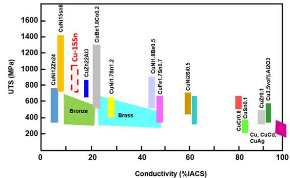
Figure 1: Strength and electrical conductivity (IACS) of Cu based alloys<sup>[6]</sup>. The goal of investigation was to achieve the UTS about 950 MPa and IACS about 18% nearly comparable to Cu-Be alloy.
