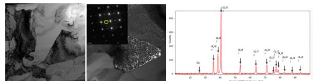
Figure 3: TEM micrographs, corresponding diffraction pattern and XRD pattern shows presence of  $Ti_3Al$  ordered structure in annealed samples.
