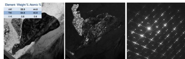
Figure 2: TEM micrographs and diffraction pattern corresponding to ordered structure.
