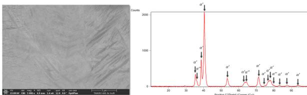
Figure 1: As built microstructure and XRD pattern. The main phases detected are, hexagonal  $\alpha'$  and orthorhombic  $\alpha''$ .
