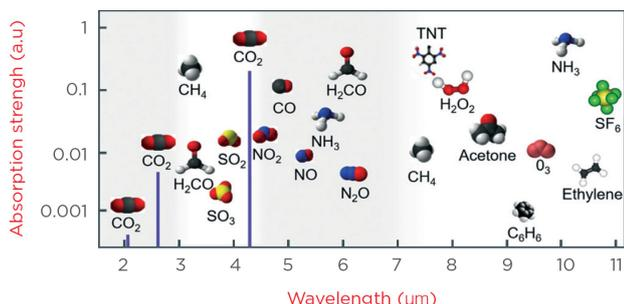
Figure 1: Absorption wavelengths and strengths of various gases.
