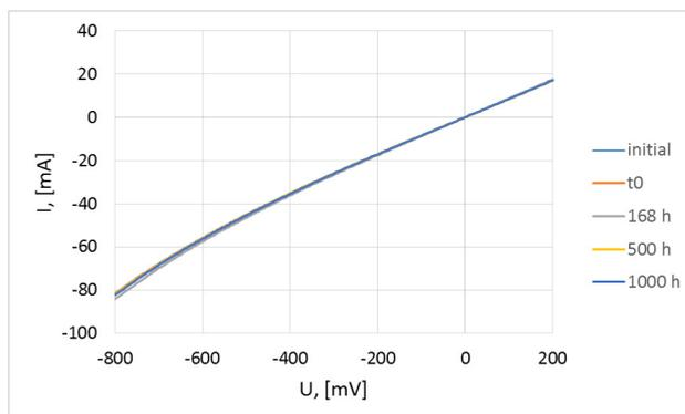
Figure 3: I-V characteristics of an IR detector subjected to T-accelerated lifetime test. A close overlap of the curves indicates no device failure.
