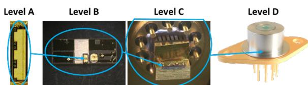
Figure 2: Integration levels of IR components (example: mid-IR laser).
