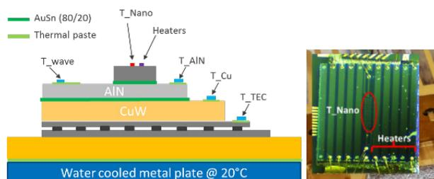
Figure 1: (left) Package configuration cross-section; (right) zoom on the heater test-chip assembled for die-attach evaluation purposes.
