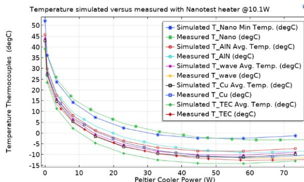
Figure 2: Thermistors temperature measured versus simulated with varying thermo-electric cooler power. Test-chip heater fixed at 10.1 W.
