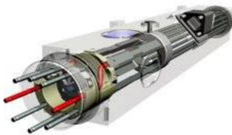
Figure 1: Draft of an "Hg trapped ion" atomic clock [1].
