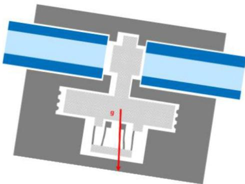
Figure 1: A concept for a Fabry-Perot optical MEMS inclinometer.
