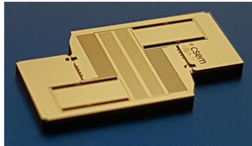
Figure 2: Fabricated silicon inclinometer chip from SOI wafer.
