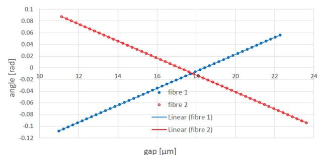
Figure 3: The linear fitting of the inclinometer calibration curve.
