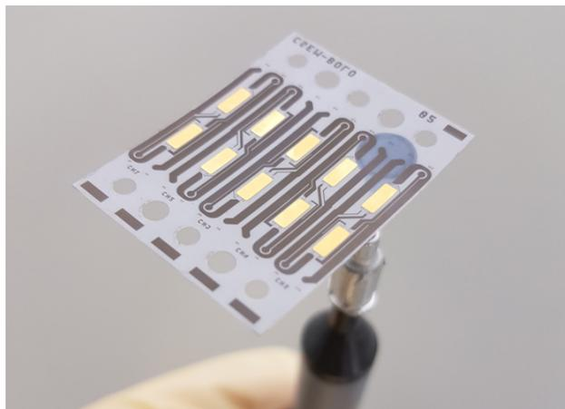
Figure 1: 5-channel bolometer sensor (25 x 33 x 0.02 mm<sup>3</sup>).
