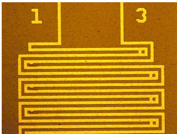
Figure 2: Detail of meanders with laser-trimmed features on the left.
