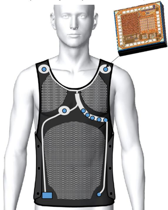
Figure 1: Drawing of the developed vest showing the sensors, conductive tracks, and pads allowing custom fine positioning of the electrodes as well as the ASIC embedded in the cooperative sensors.
