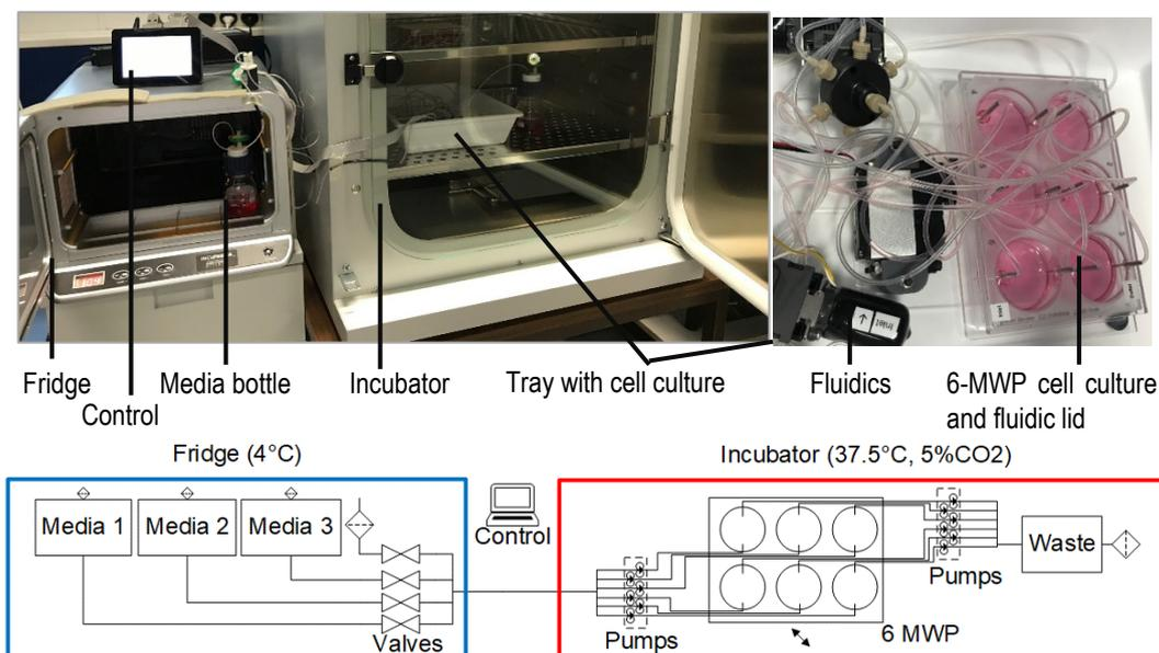
Figure 1: Automated culturing system with the buffer stored in the fridge and the cell culture in the incubator.
