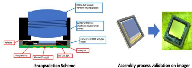
Figure 2: Encapsulation approach (left) and first tests on imager only (right).
