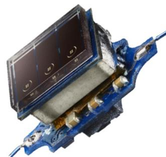
Figure 2: Photograph of the miniature wireless sensor node.
